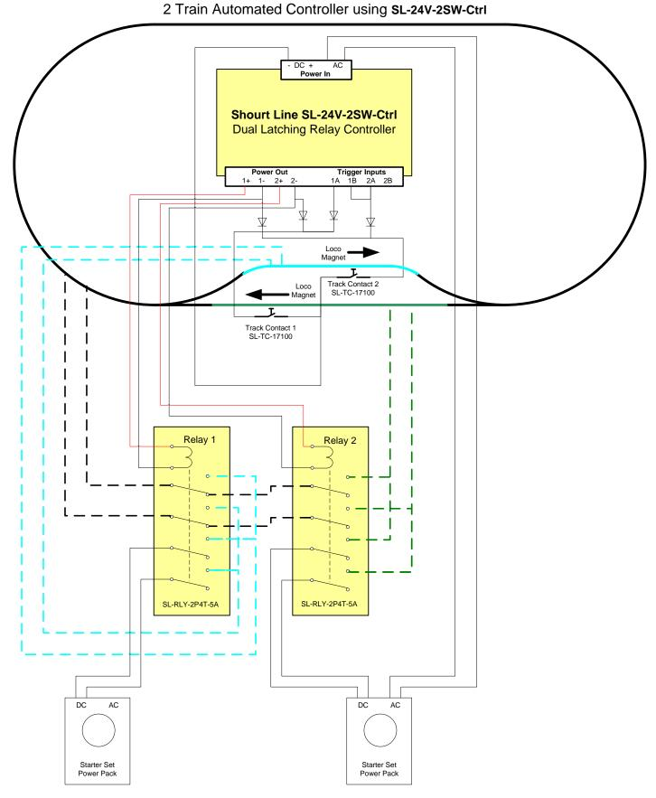
This application shows how to run two trains in opposite directions on the same track using any two power packs DC or MTS/DCC for independent speed and direction control of each train.
